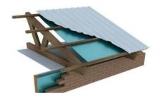
Performance Comparison of Reflecta-Guard Version 2 Plus™ to Competing Insulation Materials Flat Metal Roof 0-5° & Flat Plasterboard Ceiling Winter Insulation Break (Downwards) (Upwards) GI Building Sciences™ Reflecta-Guard Version 2 Plus™ RT 3.2 RT 1.3 0.20 2\* 60mm Glasswool Roofing Blanket RT 2.1 0.20 RT 3.5 3\* Kingspan Insulbreak 65 RT 3 2 RT 1 4 0.20
